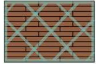
**Over 64 m<sup>2</sup>: create a grid of 4 m by 4 m with the tackifier**
